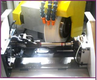
System features: **Weldon** custom 3" wide wheel guard,, Weldon custom workhead center / driver / counterbalance assembly to engage 60 degree center in end of part and drive from flange, **Encyclon** model 652-100 cyclonic coolant filtration system, **Absolent m**ist collector with HEPA filter, and **Fanuc** 0*i* TD CNC
