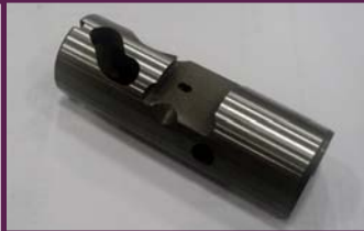
Pneumatic chuck with custom jaws
